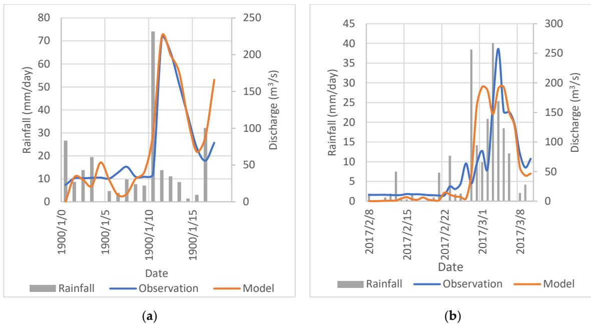
**Figure 6.** The hydrograph results of rainfall-runoff inundation modelling compare with daily observation discharge data (a) flood scenario 9 to 26 December 2019; (b) flood scenario 8 February to 10 March 2017
