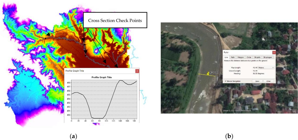
**Figure 4.** River geometry input for model RRI: (a) cross-section checking using dem; (b) river width checking using satellite images (source : Google Earth).
