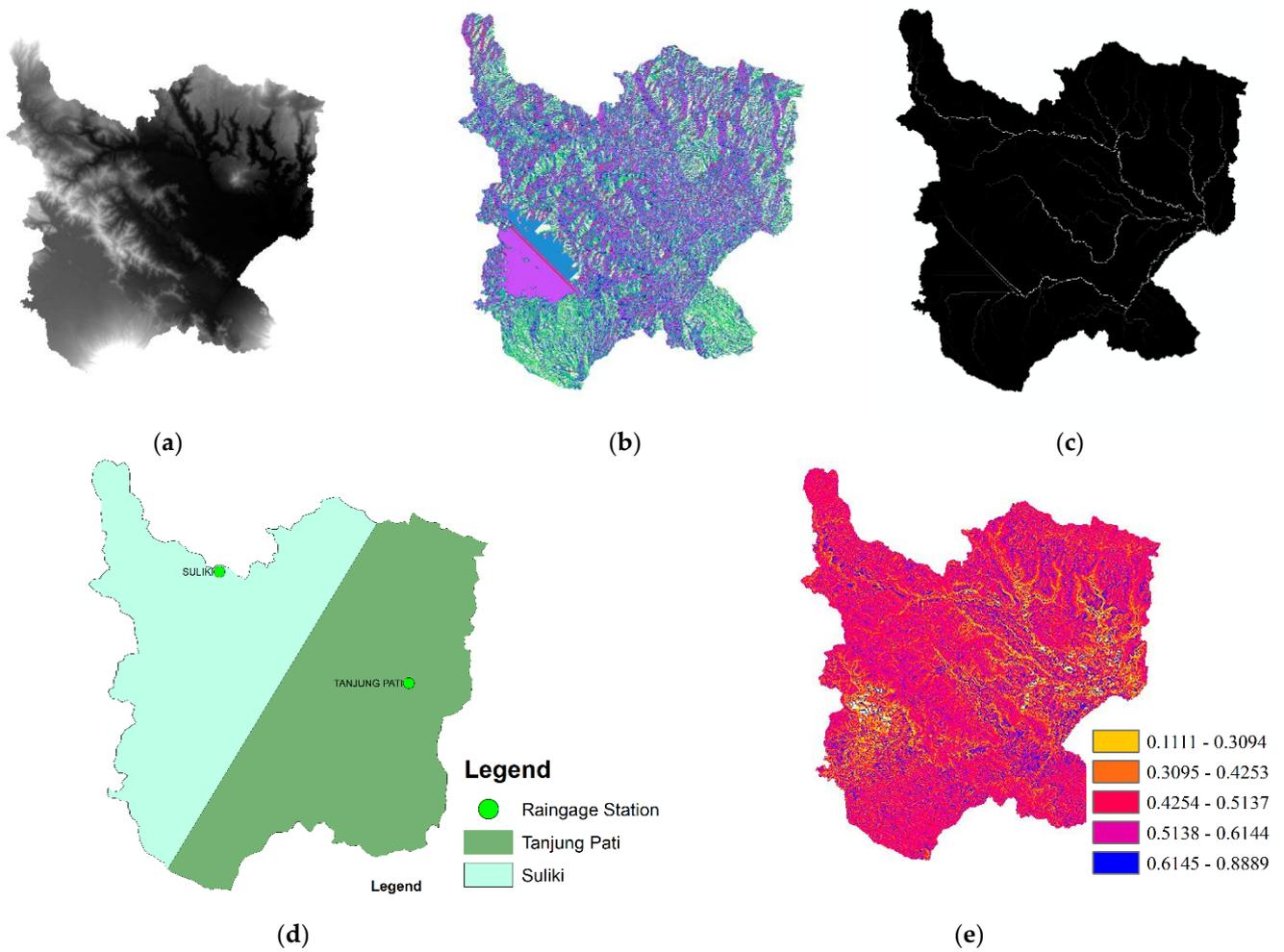
**Figure 3.** Topographic information as input RRI Model: (a) dem; (b) flow direction raster; (c) flow accumulation raster; (d) thiesen polygon area; (e) roughness coefficient
