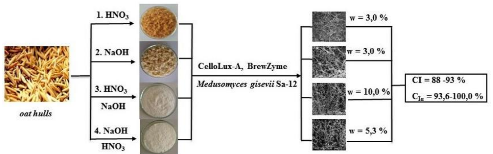
Fig. 1. Technology for the production of bacterial nanocellulose
