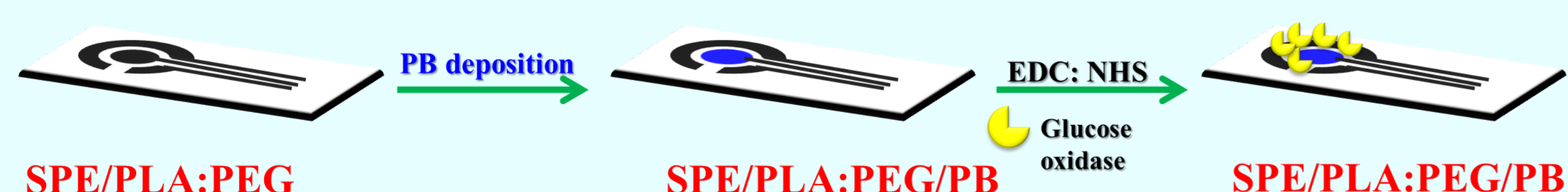
Fig 2. Fabrication principle of the bifunctional surface.
