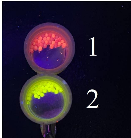
Figure 1. Fluorescent tracers under UV light. tracers based on superabsorbent polymer loaded with Rhodamine B (1); tracers based on superabsorbent polymer loaded with fluorescein (2).
