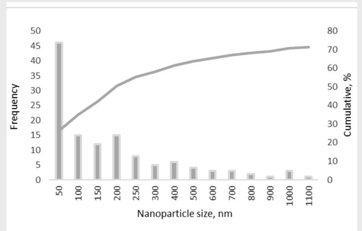
Figure 1. Size distribution of SiO<sub>2</sub> nanoparticles in DI water.
