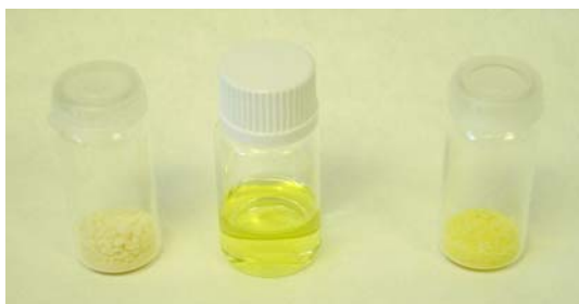
Figure 1: Gold precursor supported onto a g-SILLP before the reduction: left, SILLP; middle, Au(III) solution of HAuCl 4 ; right, Au(III) supported.
