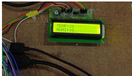
Figure 2. Photograph of the LCD display showing the real-time temperature and humidity readings.
