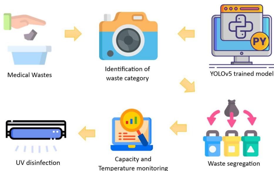
Figure 1. System design of microcontroller-based automated infectious waste segregation and disinfection system.
