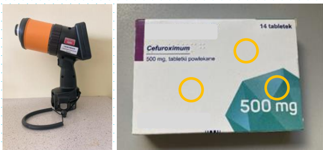
Figure 1. On the left - directional Hemispherical Reflectometer. On the right - exemplary outer cardboard package of cefuroxime drug with measurement areas within white and colored areas.
