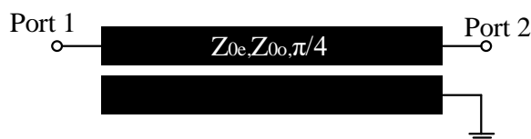
Figure 1. The band stop filter based on microstrip parallel coupled lines for microwave sensor.
