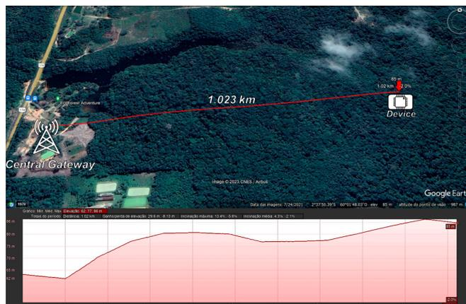
Figure 4. Validation Route for LoRa Communication Distance Between Gateway and Device, and Terrain Elevation Profile.
