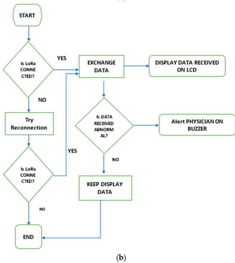
Figure 3. (a). Flowchart for LoRa Transmitter Circuit; (b). Flowchart for LoRa Receiver Circuit.
