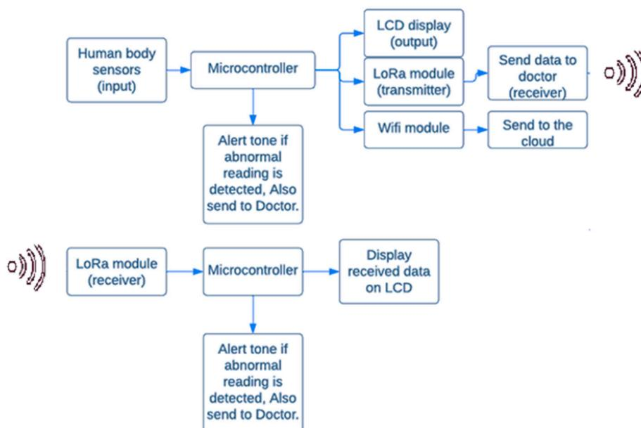
Figure 1. Block Diagram for the transmitter and receiver.
