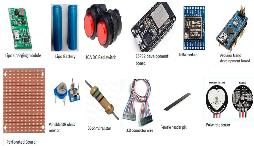
**Figure 2.** Circuit Components for the LoRa and IoT-Based Health Monitoring and Alarm System.
