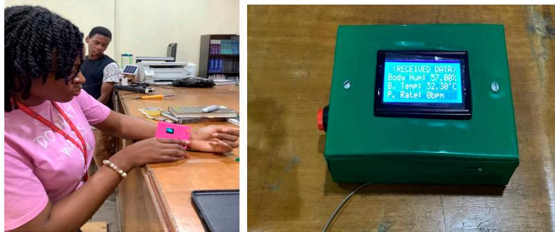
**Figure 4.** The use of the vitals monitoring prototype at the transmitter which is also displayed at the receiver end.
