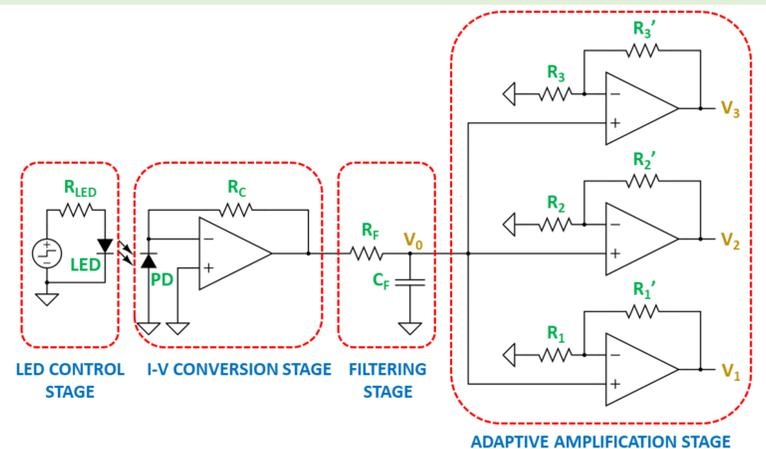
3 processing stages: (1) Low-pass filtering (to remove high frequency noise); (2) Adaptive amplification stage (to optimize the resolution of the microprocessor ADC); and (3) Digital synchronous filter (to remove low frequency noise)
