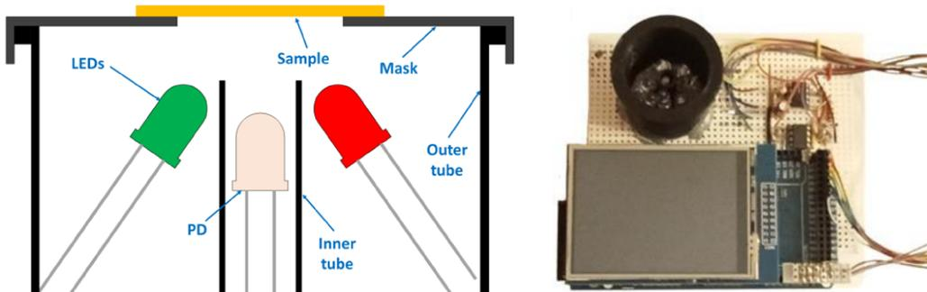
Measurements are performed on **7 bands**, from blue to near - infrared, and up to 9 vegetation indexed are computed. **Bill of materials < USD 65**.
