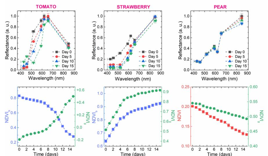
As for **tomatoes** and **strawberries** there is no significant change in the red and infrared bands, the **NDVI cannot be used** to monitor their ripening: **Instruments that only measure the NDVI are not applicable**.
