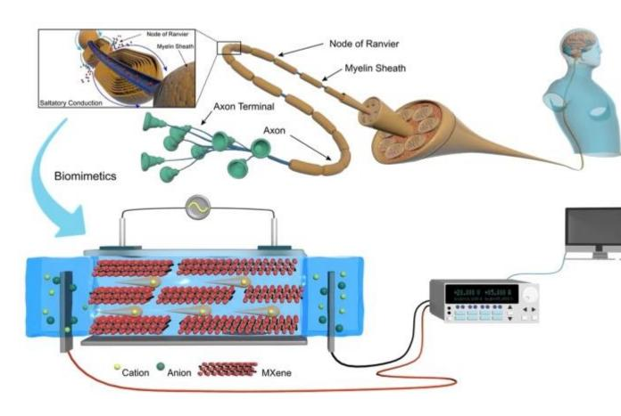
The saltatory neural conduction along axons is a unique action potential propagation pattern limited myelinated axons, to demonstrating ultrafast signal transmission. The bioinspired nervous signal transmission system is a 2D MXene nanofluidic device with signal input and acquisition modules, enabling real-time current feedback and signal transmission.
