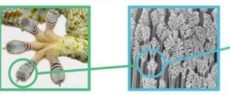
The unique geometry of our Dry Adhesive mimics the gecko's foot structure creating their signature noresidue grip. Our micro wedges replicate the soles of their feet that are covered in "hairs" called setae.
