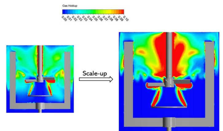
Figure 5. Variation in flow regime upon scale-up that originated the large error in the scale-up validation data ( $N_c = 280.4$  rpm;  $N_a = 18.7$  rpm, and  $Q_g = 68$  L/min).
