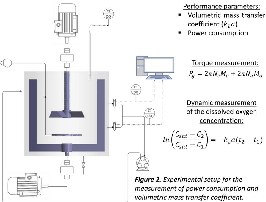
Figure 2. Experimental setup for the measurement of power consumption and volumetric mass transfer coefficient.
