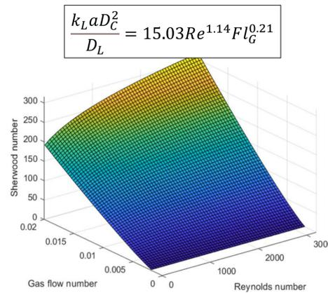
Figure 4. Estimated effect of gas flow number and Reynolds number on the dimensionless volumetric mass transfer coefficient.
