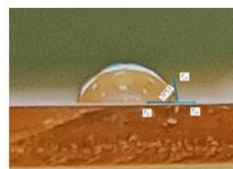
Figure 5. The edge angle of wetting with water
