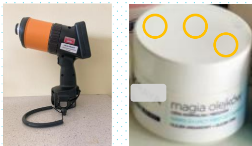
Figure 1. On the left - directional Hemispherical Reflectometer. On the right - exemplary white plastic package of moisturizing creams with measurement areas within a plastic container.
