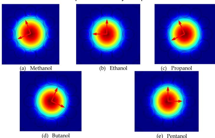
Figure 3. Electromagnetic field distribution for different alcohol analytes.
