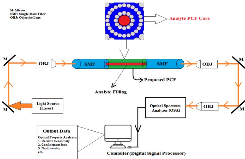
Figure 2. Schematic representation of proposed MC-PCF refractive index sensor integrated photochemistry setup.
