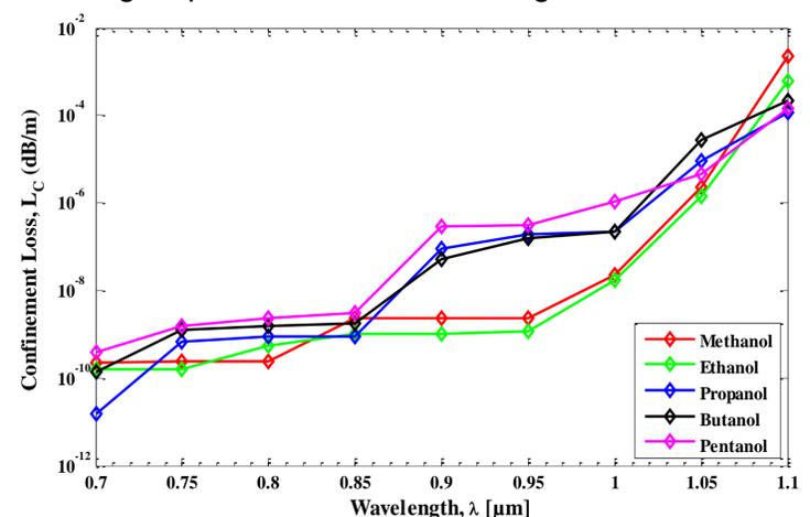
Figure 6. Wavelength versus Confinement loss curve for different alcohol analytes.
