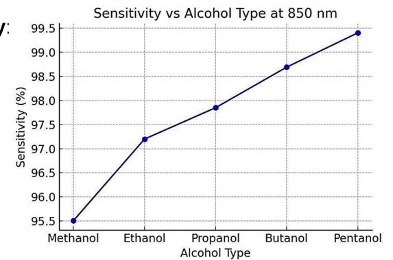
Figure 4. Plot of Sensitivity vs. Alcohol Type at 850 nm
