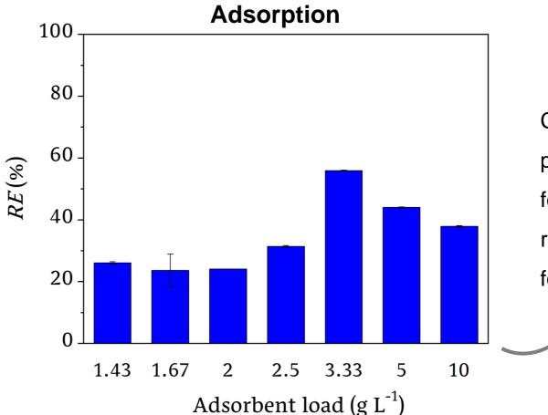
CuFe LDH was tested towards the Clphe, in **adsorption** with varying loads for **24 h**. This test showed an ability to remove **56%** of the Cl-phe (**10 mg/L**), for a load of 3.33 g L<sup>-1</sup>.
