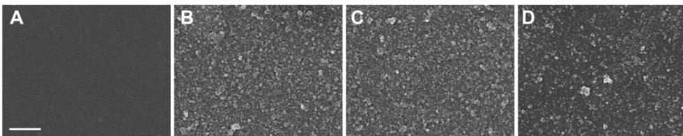
Figure 1. SEM images of (A) GS-OH, (B) GS-NH<sub>2</sub>, (C) GS-TPCF<sub>20</sub>, and (D) GS-ZnTPCF<sub>20</sub> surfaces (scale bar 400 nm).
