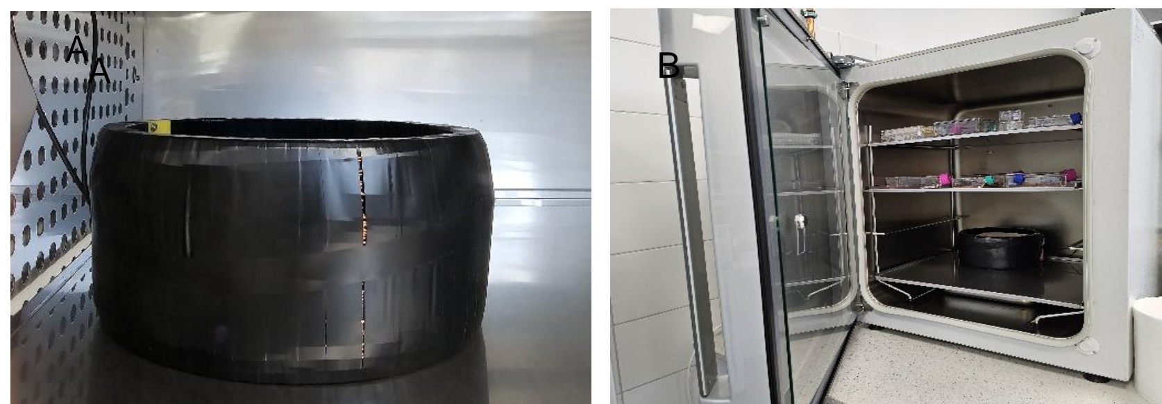
Fig.2. View of the designed solenoid (a) and the inside of the incubator with cultures of control cell lines and cells exposed to magnetic induction in the solenoid (b)
