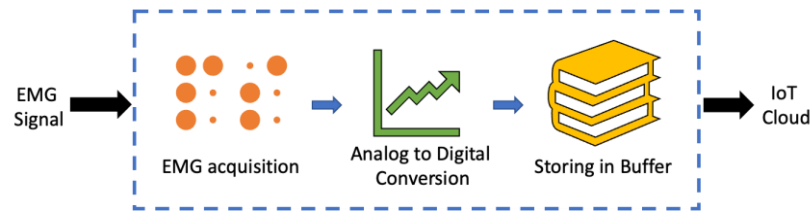
Figure 2. Function of Node MCU microcontroller.
