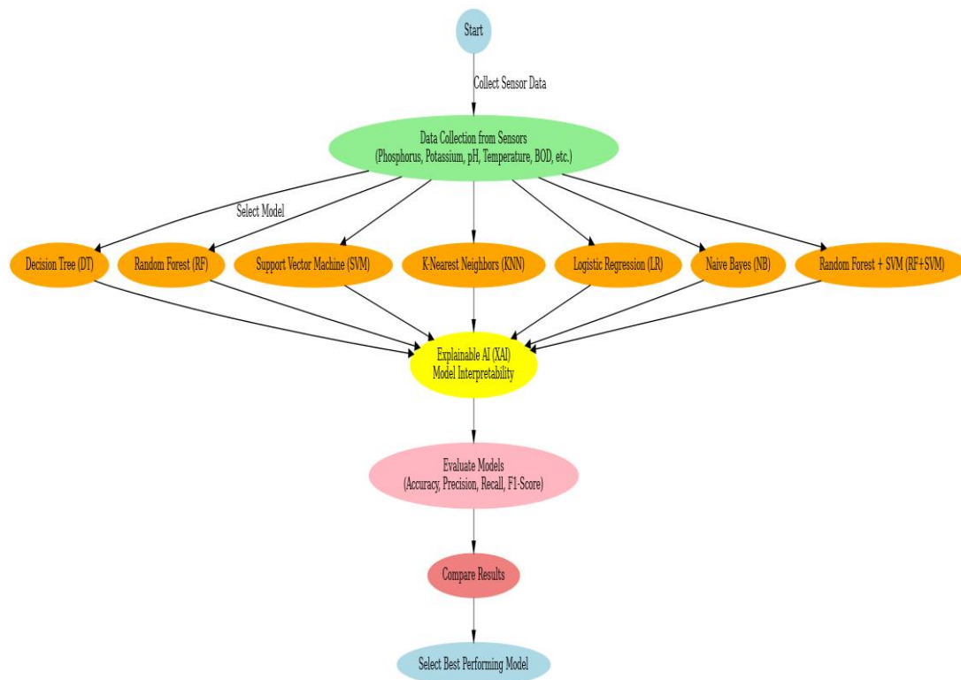
Figure 1. Proposed model for Real-Time Multi-Nutrient Water Quality Analysis in Agriculture
