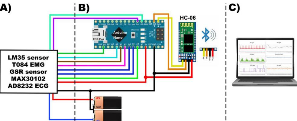
Fig. 1. Biosignal acquisition system connection diagram.
