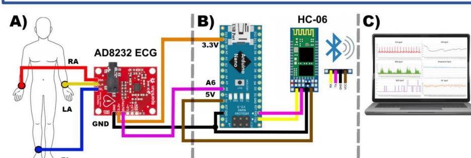
Fig. 3. ECG acquisition module diagram.
