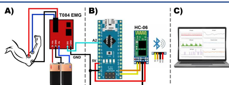
Fig. 4. EMG acquisition module diagram.
