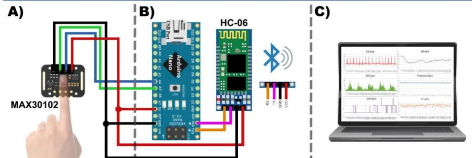
Fig. 5. HR and SpO2 module diagram.
