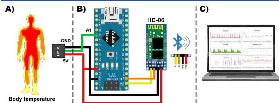
Fig. 2. Body temperature module diagram.
