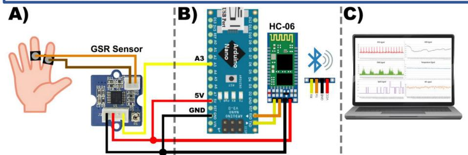
Fig. 6. GSR acquisition circuit module.
