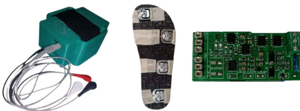
Figure 1. Photographs of the basic devices we produced within the scope of the project (left) The main device connected to the foot, the EMG cables coming out of it are visible. (mid) Measuring slippers with force sensitive resistors placed underneath, which we use for ground reaction force measurement. (right) PCB that we produced
