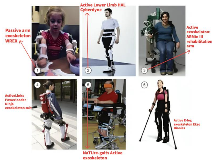
Figure 1. Examples of exoskeletons for various functions: (1) Passive arm exoskeleton WREX, (2) HAL from Cyberdyne, Japan, (3) ARMin III rehabilitation arm, (4) ActiveLinks Powerloader Ninja exoskeleton suit, (5) NaTure-gaits, and (6) E-leg exoskeleton from Ekso Bionics.
