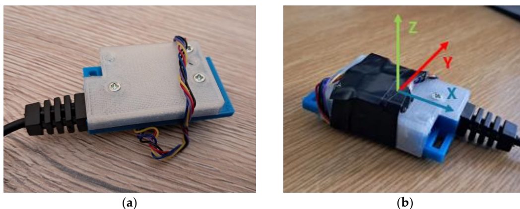
Figure 1. Prototype inertial measurement units of the sensor, which is stored in a package with handles for possible fixing (a) and the sensor with axes marked in the X, Y and Z directions (b).
