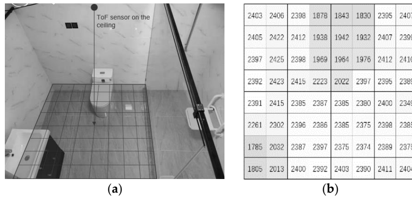
Figure 5. (a) Experimental setup with ceiling-mounted ToF Sensor; (b) A representative single-frame output of ToF the sensor.
