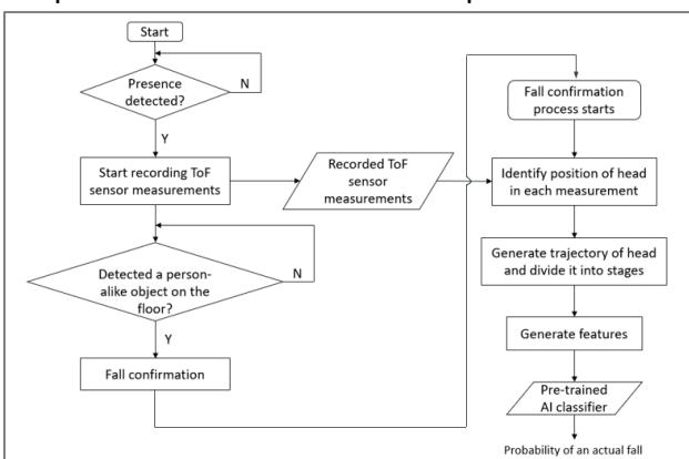
Figure 2. Workflow of the fall detection system.
