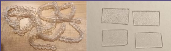
Fig.1. (a) Clear aligners. (b) Flat samples were cut after thermoforming the PET-G sheets.
