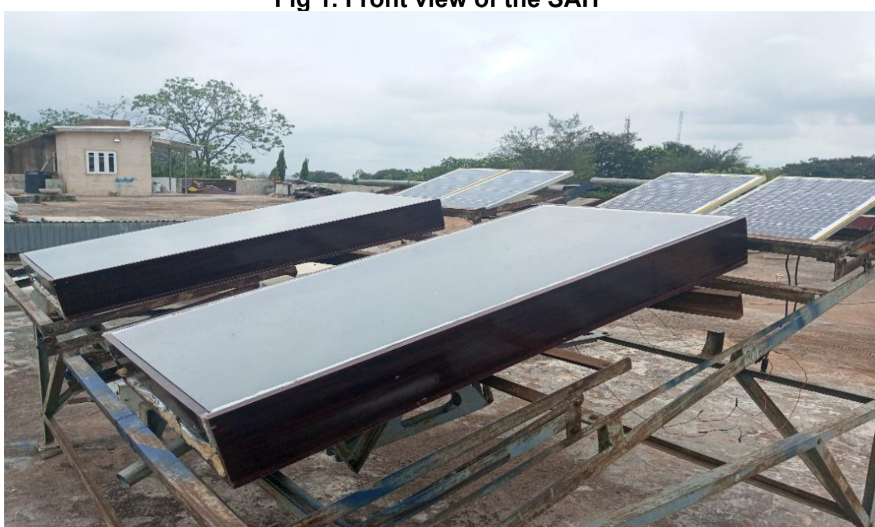
Fig 2. Pictorial view of the two prototype SAHs during testing
