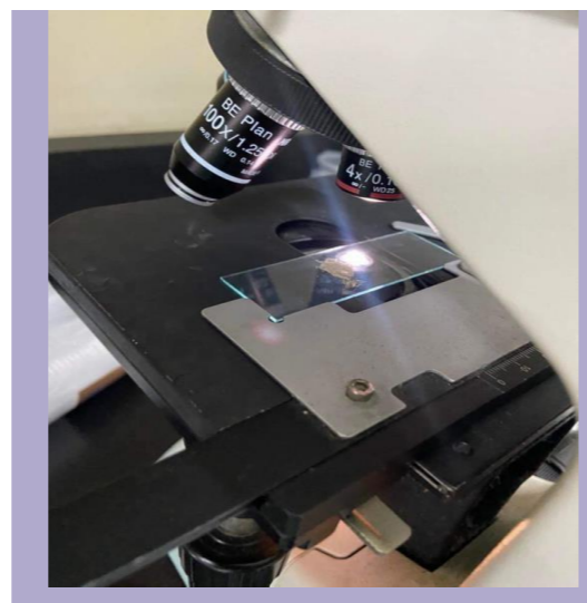
Fig 5. Visual inspection for identifying microplastics using a microscope.
