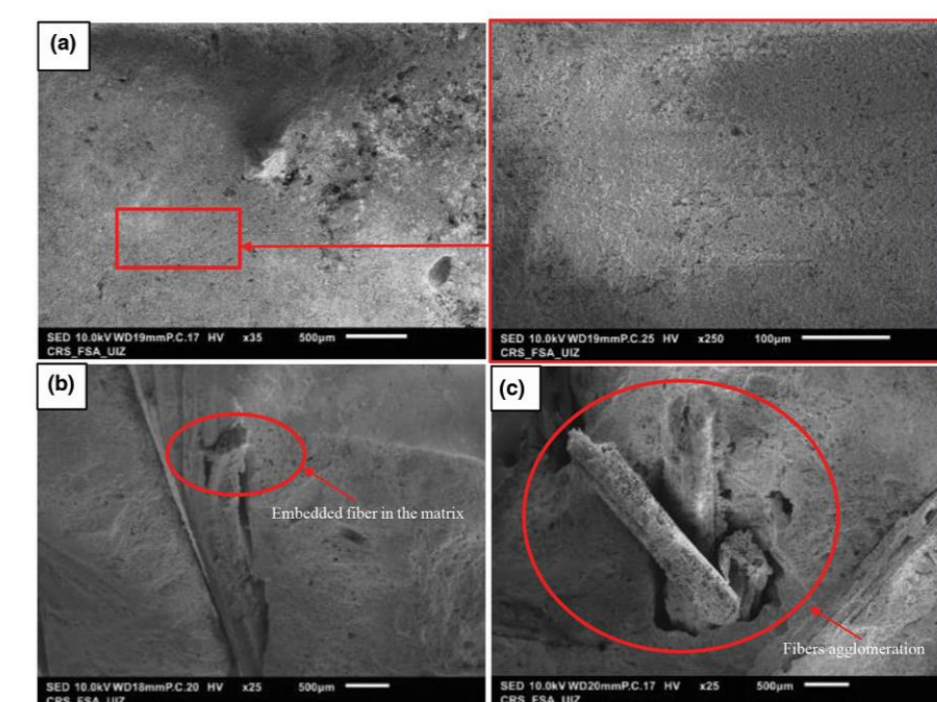
Fig.15: Secondary electron SEM images of the fracture face, (a) plaster, (b) plaster composite incorporated with 20% JM fibers, (c) plaster composite incorporated with 40% JM fibers
