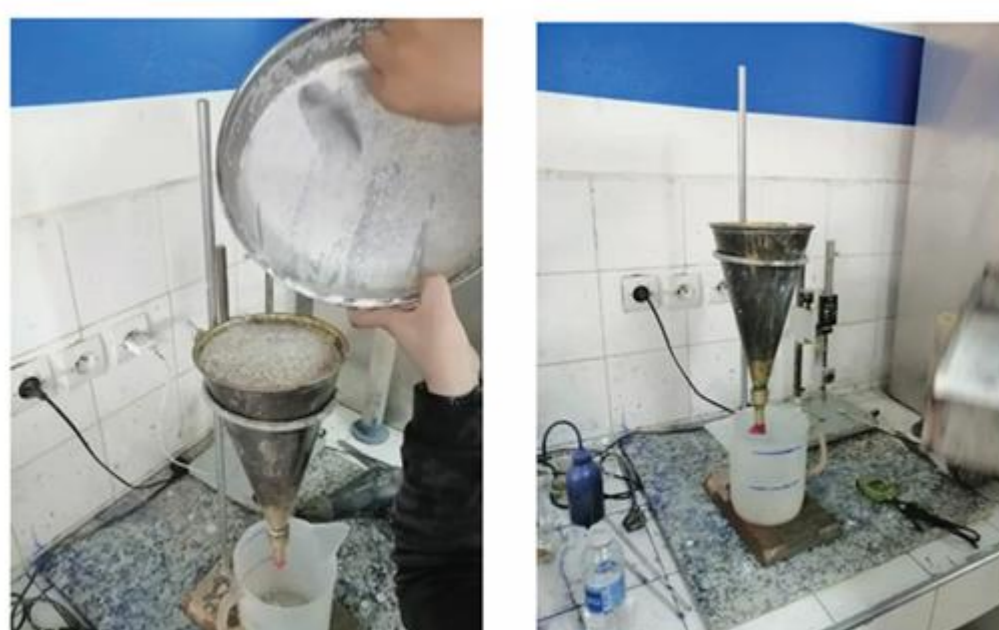
Fig.7: Manipulation of Marsh cone on the plaster paste incorporated by JM fibers
