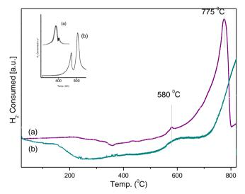
Figure 3: TPR diagram between ambient T and 820 °C for the phases: (a) MnMo9 and (b) MnMo9/Diat.
