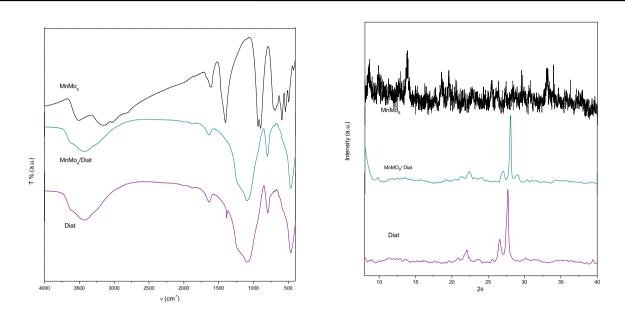
Figure 2: A) Comparative FTIR spectrum of  $MnMo_9$ , diatomaceous earth and  $MnMO_9$  supported on diatomaceous earth and B) DRX comparative
