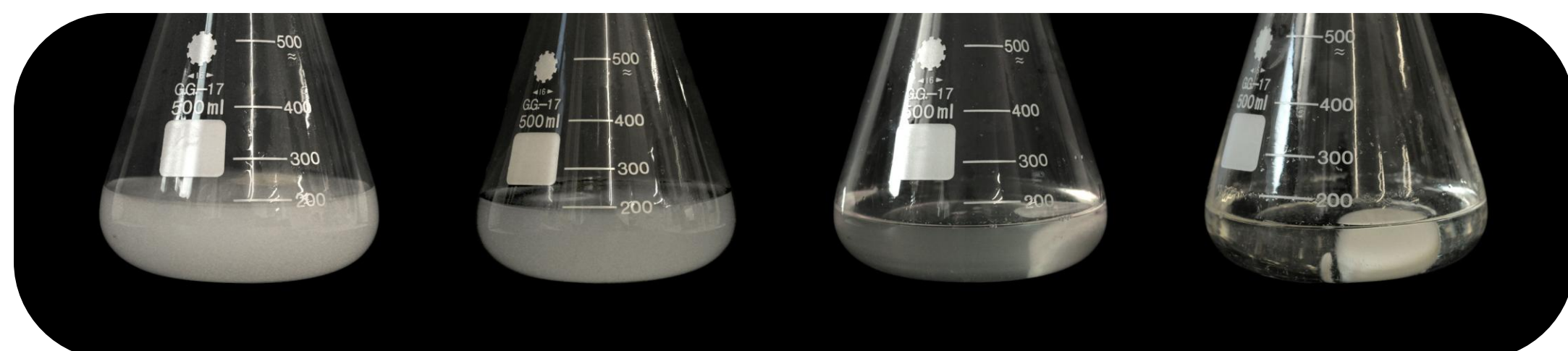
Visual progression of Impranil® DLN-SD degradation from day 0 (opaque) to day 10 (fully transparent)
