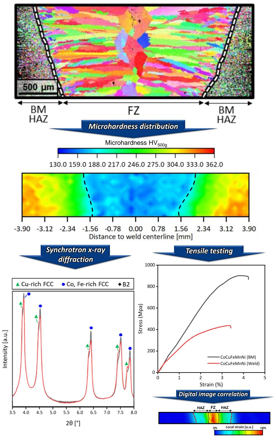
**Aim:** To evaluate the feasibility of gas tungsten arc welding on the CoCuFeMnNi high-entropy alloy by analyzing its microstructure and mechanical performance across the welded joint.
