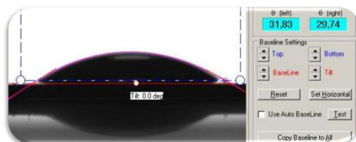
Distribution of water droplet on the surface of the graphene sample after treatment in acid medium
