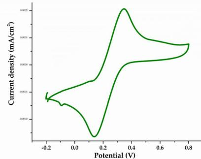
The CV of curve one cycles was taken from -300 mV to 900 mV vs. Ag/AgCl with a scan rate of 100 mV/s of graphene@Au sample in 2.5 mM [Fe(CN)<sub>6</sub>]<sup>3-/4-</sup> in PBS (pH 7.4) electrolyte.
