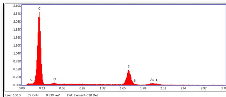
EDX spectrum for a representative sample of graphene decorated with gold nanoparticles
