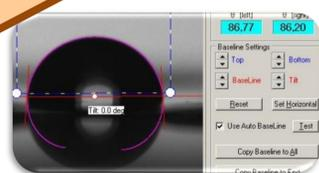
Water droplet distribution on the surface of the graphene sample
