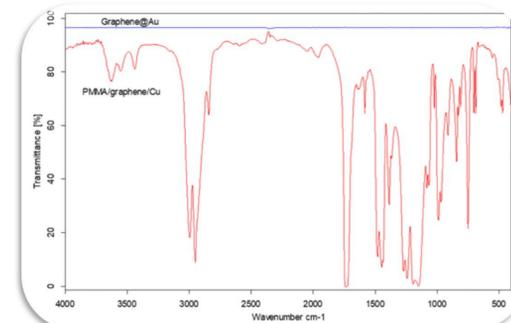
FTIR spectra for the graphene sample before transfer onto the SiO<sub>2</sub> substrate, after modification of wetting capacity and decorated with gold nanoparticles
