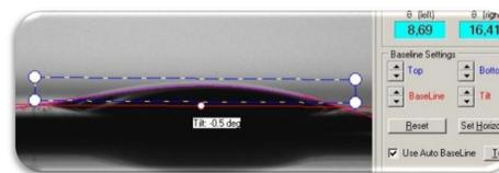
Water droplet distribution on the surface of the graphene sample after plasma treatment
