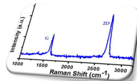
Raman spectrum of the graphene sample after plasma treatment
