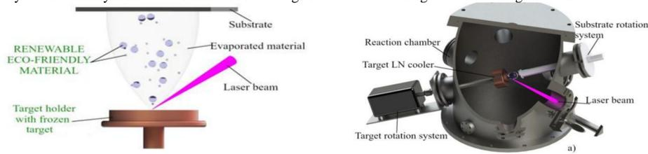
Matrix Assisted Pulsed Laser Evaporation (MAPLE) experimental set-up and mechanism.
