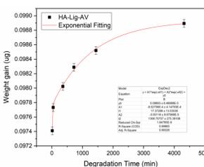
Weight gain,  $\Delta m$ , as a function of immersion time in SBF(15 min, 45min, 2h, 6h, 12h, 72h).
