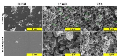
SEM micrographs of HA-Lig and HA-Lig-AV2 samples, deposited initially and at different degradation time intervals (15 min and 72h).
