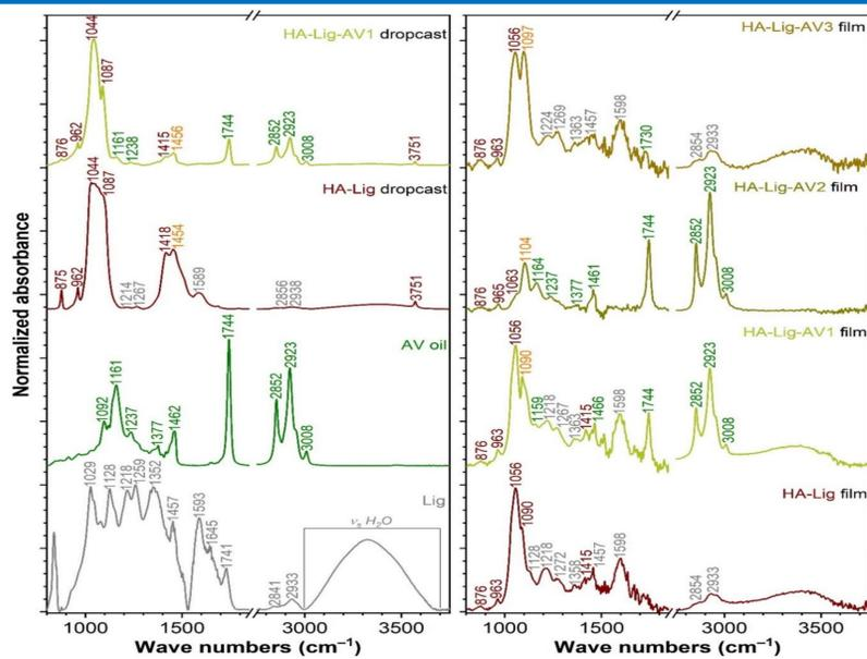
FTIR spectra of the investigated materials: Lignin powder; Aloe Vera essential oil, HA-Lig (dropcast and thin film); composite films: HA-Lig-AV1 (dropcast and thin film); HA-Lig-AV2 thin film; HA-Lig-AV3 thin film.
