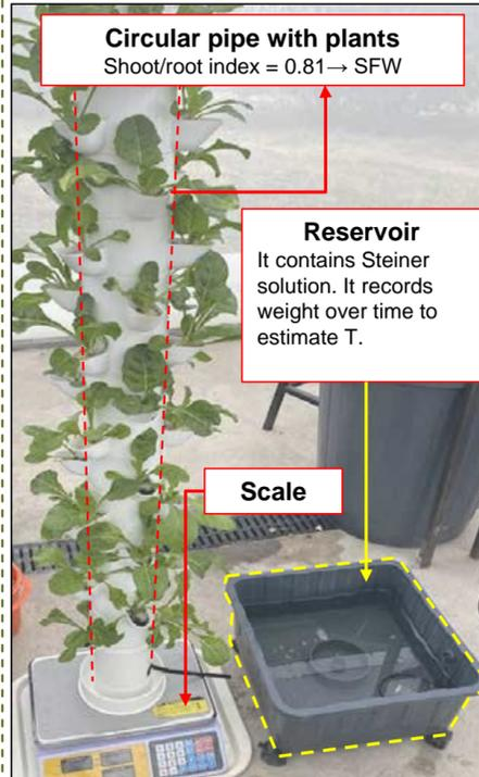
**Figure 1.** Weighing process to estimate the shoot fresh weight and transpiration of a vertical hydroponic tower.
