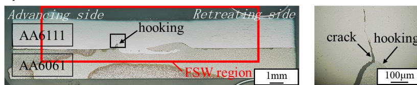
(a) Cross-sectional image. (b) Fatigue crack. Figure 1. Cross section of the fatigued FSW joint.
