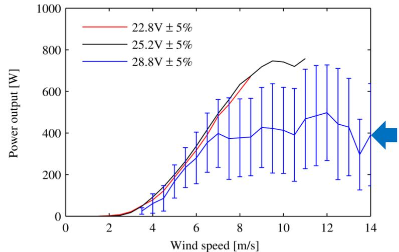
Following IEC standard, the systems includes the charge controller and the dump load. The charge controller is connected in parallel to the generator rectified output. It diverts the energy to the dump load when the battery voltage rises above a preset level (26.4 V here). This happens when the battery is fully charged or during wind gusts. The resulting effect can clearly be seen on the  $28.8\text{V} \pm 5\%$  power curve: the output power has a large standard deviation and drops in average.
