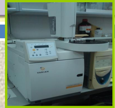
Fig. 3.2. Varian 430-GC, connected to a HT5 capillary column with a flame ionization detector (FID) at 450 °C and splitless injection at 350 °C. Helium is used as carrier gas, with a flow of 1.5 ml/min. It has been applied a heating ramp from 90 °C to 200 °C at a rate of 7 °C/min, followed by another ramp from 200 °C to 360 °C at a rate of 15 °C/min, maintaining the temperature of the oven at 360 °C for 10 minutes.
