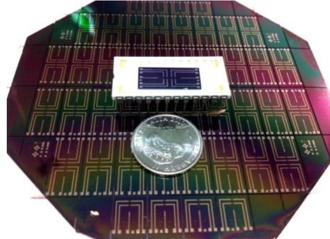
A novel wafer-scaled top-down process for the fabrication of locally thinned-down silicon nanowires based device has been developed
