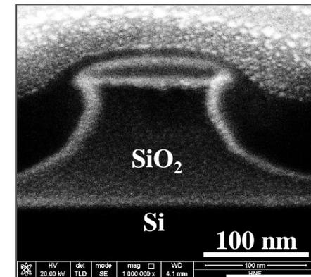
Ultrathin SiNWs were fabricated with thickness down to ~20 nm by localized wet-etching with optimized TMAH
