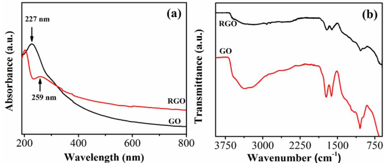
UV-vis spectroscopy and FTIR confirmed the reduction of graphene oxide
