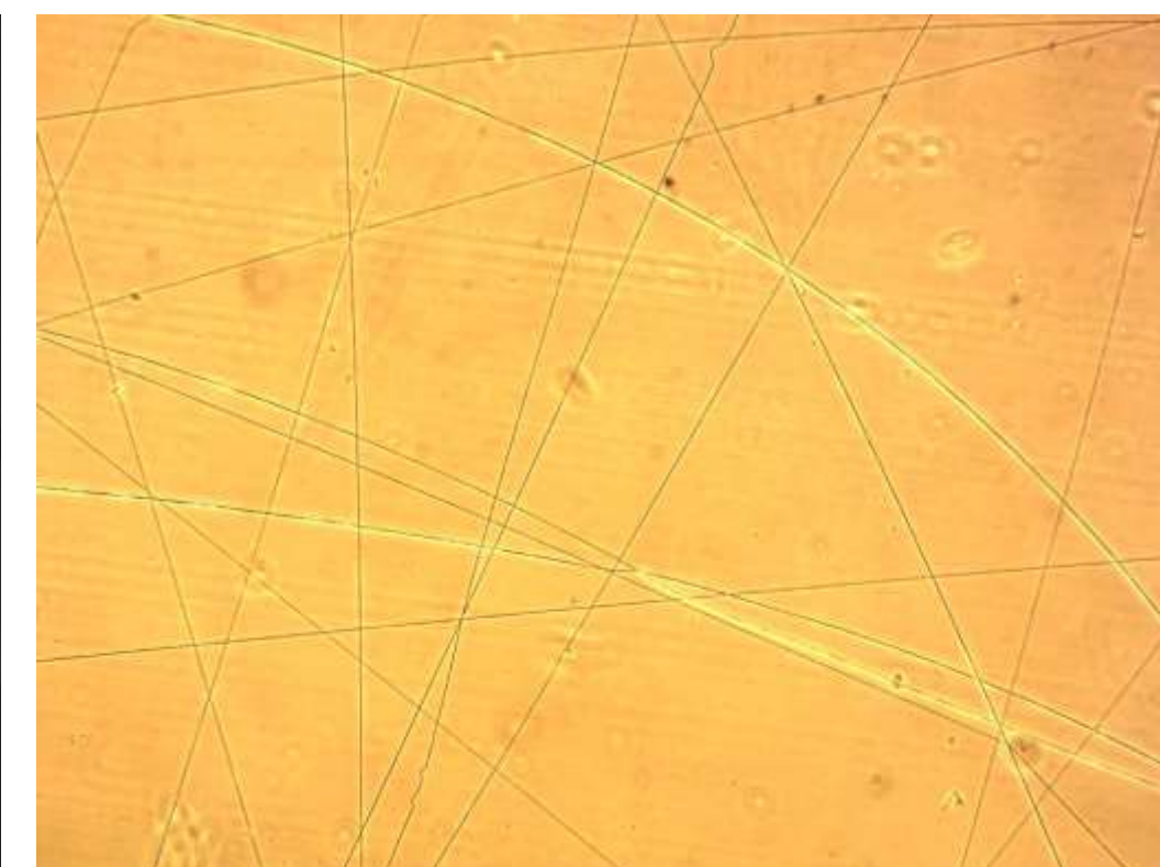
Figure 3. SA/PEO fibers under optical microscope
