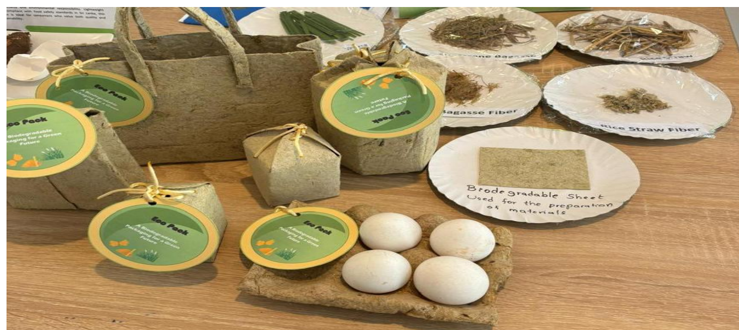
Figure 02: Prepared materials for several applications with P3 (SB : RS : CGL = 1:3:2) formulation
