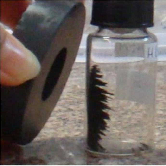
Figure 1: Magnetite catalyst obtained from the reaction of Fe 2+ ions and OH - ions, exposed in the magnet field of a magnet
