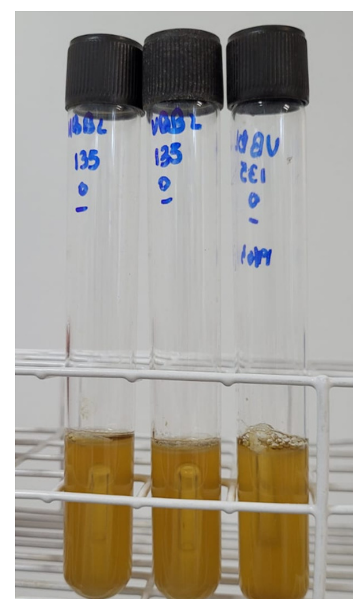
Figure 2. Brilliant Green Bile Lactose broth tubes with gas formation in the inverted Durham tubes, confirming the presence of total coliforms.
