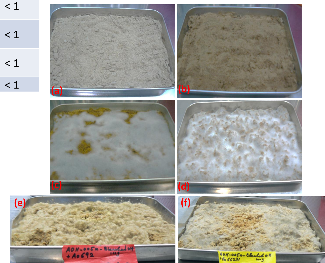
Fig.5. Static SSF on milled oat hulls. (a). Pre-inoculation, (b). Post-inoculation with inoculum density at CFU = 1 E+07 per 100 g substrate with moisture adjusted to 50%, (c). Mycelial growth on surface of substrate after three days, (d). Mycelial growth on surface of substrate after seven days, (e). Inoculated with A. oryzae , (f). Inoculated with R. oligosporus
