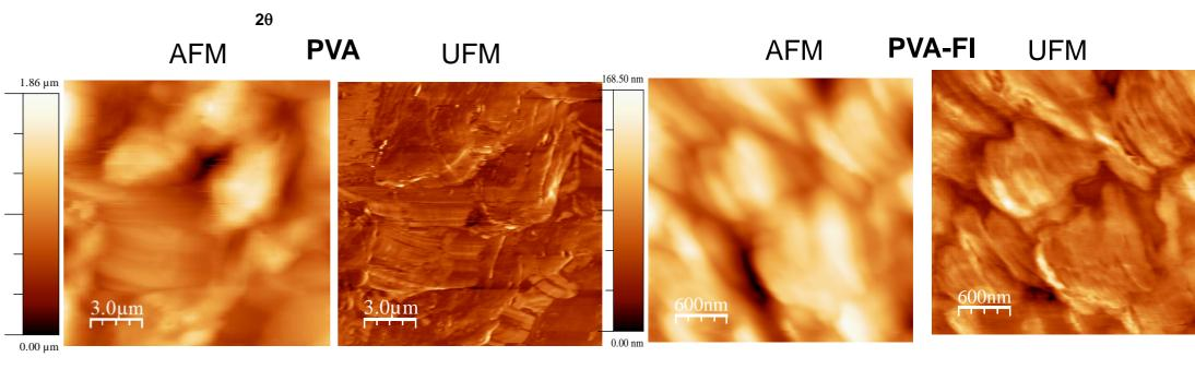
On both PVA and PVA-FI samples the topography is characterized by a patch-liked layered texture typical of FDM. Smaller patches were better resolved in the PVA-FI sample. On both samples, UFM reveals nanoscale elastic inhomogeneities, which may arise from local density variations and/or residual interfacial stresses, and in the case of PVA-FI, also from fluorescein aggregates.
