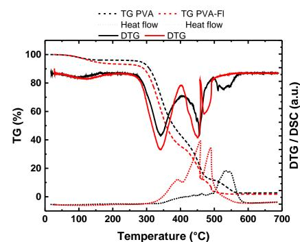
PVA-FI: slightly reduced thermal stability, modified DSC transitions ⇒ Fluorescein alters PVA thermal degradation[3].
