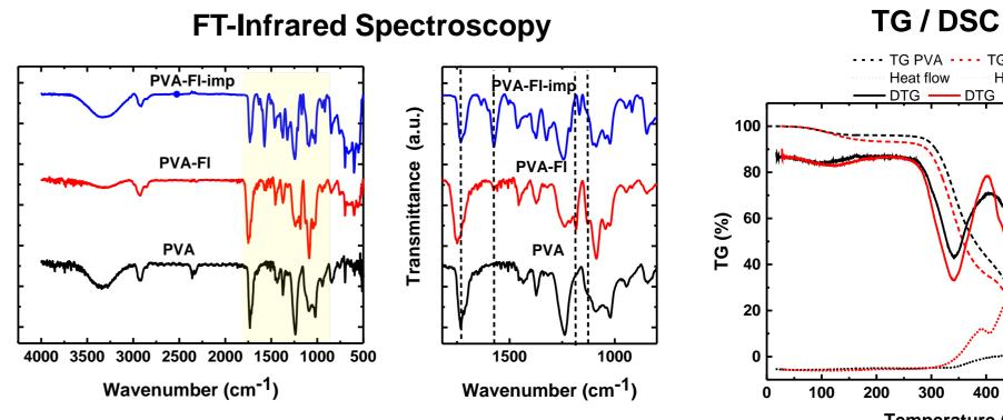
Appearance of fluorescein-related bands in modified samples. PVA-FI: peak shifts indicate PVA-fluorescein interactions (hydrogen bonding)
